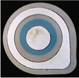
first planar transistor (1959)
